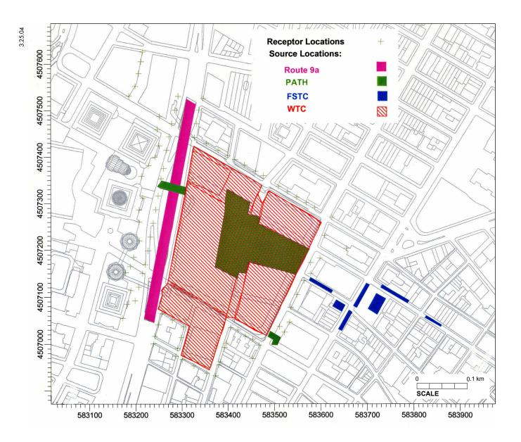
Location of Sources and Receptors in the Construction Site Air Quality Model Figure 21-32
